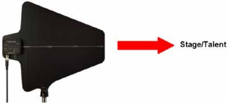
**2. Using RF booster amplifiers for the receiver antenna system gives greater operating range.** The only reason to use RF boosters in an antenna system is to overcome signal losses in the antenna cables. To determine if boosters are even needed, consider that directional antennas have about 4 dB of passive gain. Using a low-loss cable such as Belden 9913F7 means that even for a 100-foot run, there is only about 3 dB of loss at 600 MHz. Thus, a booster is not needed.
