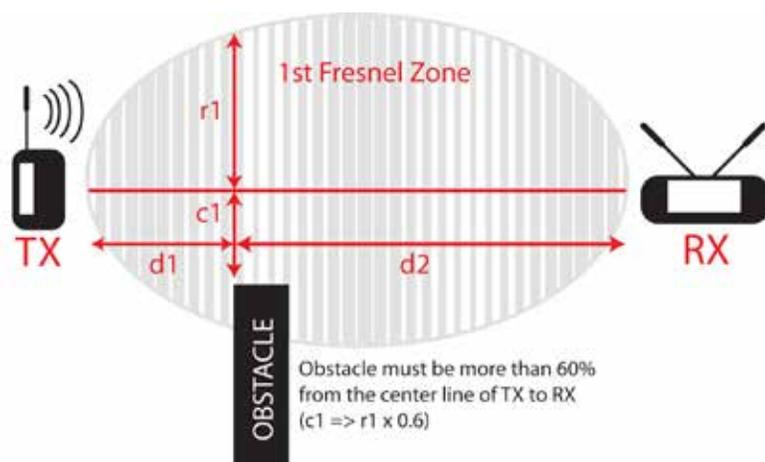
**5. Locate receivers and antennas as close to transmitters as possible.** This is like microphone technique: it's all about signal to noise. The noise floor is relatively constant, although there can be localized noise sources, too. By placing antennas close to the desired source (transmitters), you're increasing the desired signal over the undesired. Just watch out for antenna cable loss.
