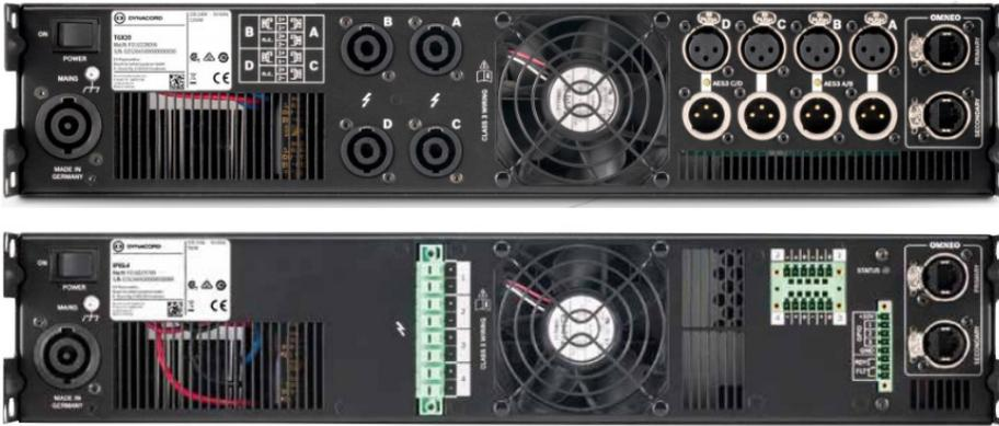
*The back panel connectors of Dynacord TGX and IPX amplifiers.*
